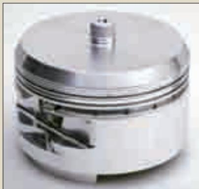
There are many other detail machining operations that may be required, depending upon the needs and specifications of the application or of the engine builder in a custom application. Here, the piston has been machined for pin retention, and lateral gas ports have been added.
