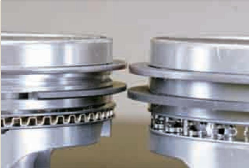
A very aggressive ring package is also part of the Pro-Series theme. The 1.2-1.5-3mm ring package is low on drag and high on conformability and is at home at high rpm. Note the comparison to the conventional 1/16-1/16-3/16 rings on the piston to the right.
