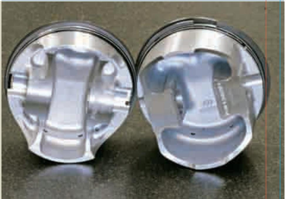
A peek under the skirt of the new Pro-Series SRP piston next to a conventional forging (right) shows the dramatic difference in design. The new piston takes its cues from JE's racing piston development.
