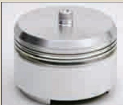
Piston-lathe operations produce the piston's basic form, the ring, attenuator, and reservoir grooves. The lathe operations are the initial step in converting a raw forging into a useable piston.
