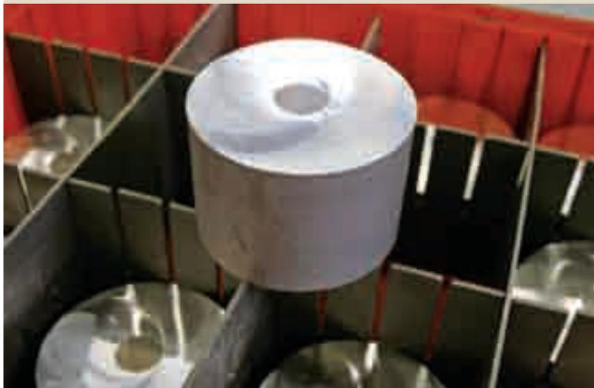
As a part of its rigorous development process, JE/SRP Pistons manufacture billet pistons from solid pucks of aluminum for dyno-testing in actual engines prior to approving the final forging designs. Testing in this way gives it an opportunity to make small adjustments to the design, improving performance and strength before adding to the product line. Actual testing allows JE/SRP to validate and verify its products' performance.
