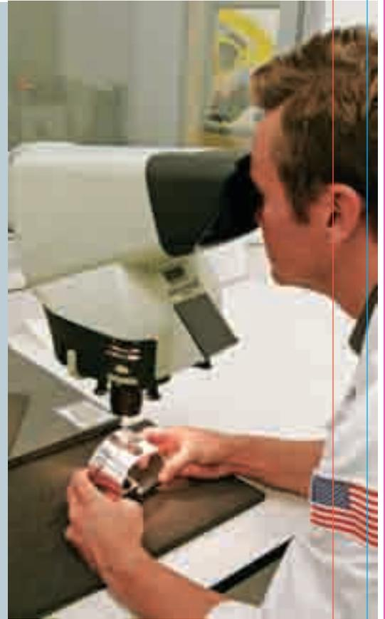
In addition to quantitative inspection, detailed qualitative inspections are also part of the program. Here, a piston is being visually inspected under high magnification for signs of machining distress and other flaws.
