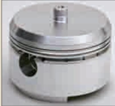
Machining the pin bore, draining oil in the ring groove, and getting the pin oilers comes next. The pin bore's position is a major aspect in matching a piston to a specific compression height and engine application.
