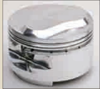
The dome profile can be as simple as a flat-top or as narrowly focused as a specific profile designed for a cylinder head's combustion chamber. Note the substantial material removal from the previous step.
