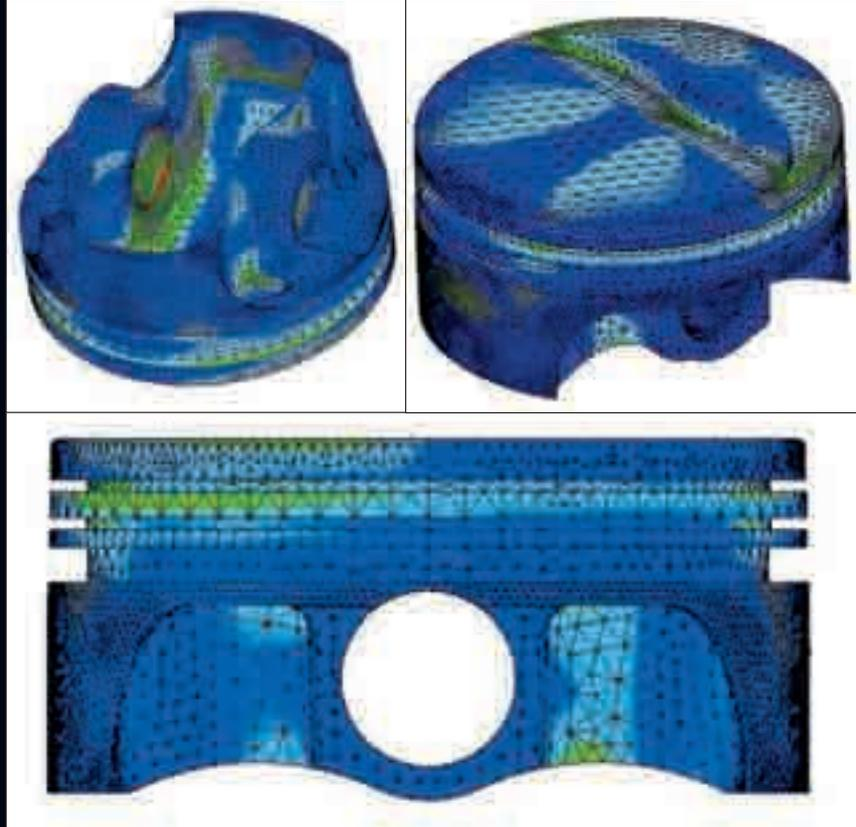
Development of the new Pro-Series SRP piston line took place over the course of an entire year. The piston designs were created using 3D computer modeling and tested for strength using Finite Element Analysis (FEA). Computer modeling using FEA technology gives a very clear indication of the stresses and forces acting on the piston under various load conditions. Continual revisions were made in the design process to optimize strength and weight before manufacturing began.
