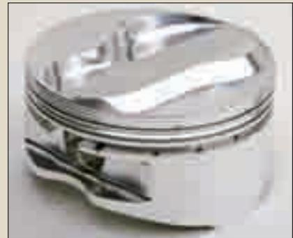
Next, the lower profile is cut away to the final shape, and the basic piston is completed. Several more machining operations can be specified depending on requirements. Deburring and cleaning finish the pistons, and then the set is boxed and ready to ship.
