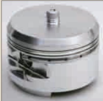
Another machining operation cuts the piston's side reliefs. This is a piston forging designed with a conventional-style skirt in mind. The new Pro-Series skirt requires a special forging and results in a different skirt configuration.
