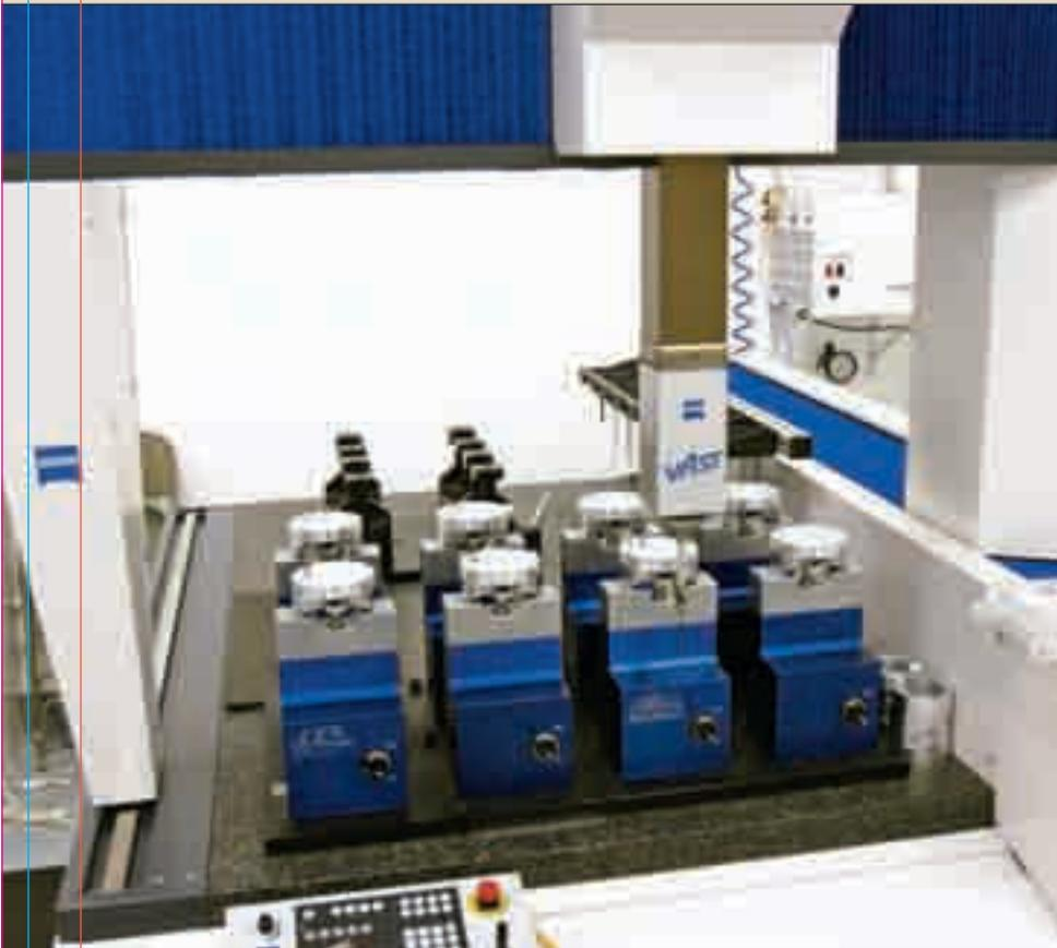
At the JE/SRP facility you will find an inspection and quality control lab that is second to none. There are numerous machines that will take highly precise quantitative measurements to ensure the pistons are right on spec.
